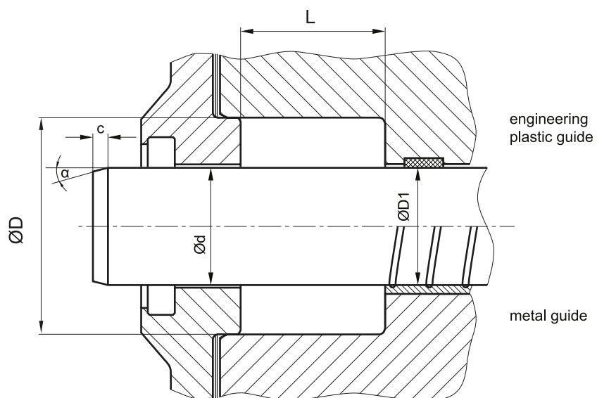
the adjustment range of the mounting space height (L) should correspond to approx. 10% of the theoretical mounting length.
