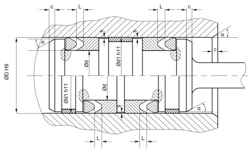
plastic guiderings (wearbands) have to feature a adequate cutting gap (recommendation: 2-5% of D). if metalic guides are used, spiral grooves shall be provided. in order to avoid drag pressure built up in case of back-to-back arrangement, the distance between the seals should be as small as possible.
