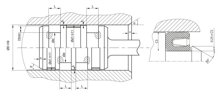
plastic guiderings (wearbands) have to feature a adequate cutting gap (recommendation: 2-5% of D). if metalic guides are used, spiral grooves shall be provided, small values for Hmin allow slipping the seal over the piston, but the height of the retaining collar has to be sufficient to assure a stable fit in the housing (see "mode of installation"), in order to avoid drag pressure built up in case of back-to-back arrangement, the distance between the seals should be as small as possible.
