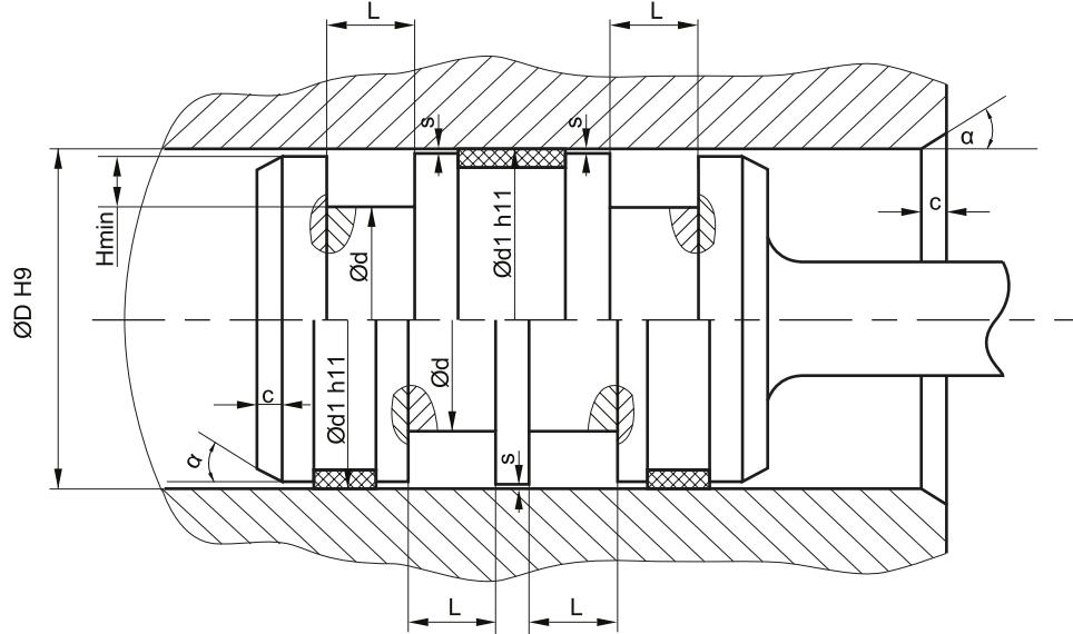
plastic guiderings (wearbands) have to feature a adequate cutting gap (recommendation: 2-5% of D). if metalic guides are used, spiral grooves shall be provided. the height of the retaining collar has to be sufficient to assure a stable fit in the housing (larger than cs/2, smaller retaining collars will increase the danger of eversion of the profile in case of occuring drag pressure).
