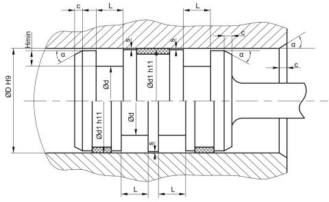
plastic guiderings (wearbands) have to feature a adequate cutting gap (recommendation: 2-5% of D). if metalic guides are used, spiral grooves shall be provided. smaller values for Hmin will ease the installation (reduced elongation and mounting force) but the height of the retaining collar has to be sufficient to assure a stable fit in the housing (larger than cs/2, smaller retaining collars will increase the danger of eversion of the profile in case of occuring drag pressure).
